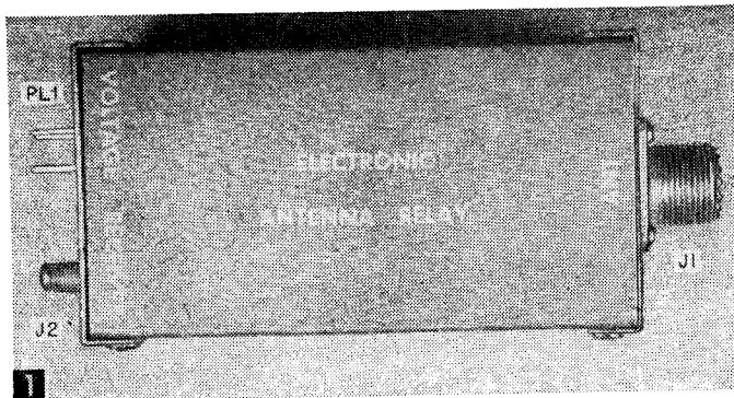
The completed electronic antenna relay, or T-R Switch, with the cabinet lid in place (above). This unit will permit instant break-in operation with CW transmitters of up to 100 watts input. It can also be used with phone transmitters running up to 85 watts. Interior of the relay cabinet showing construction and layout (below). The 6C4 is mounted on a small aluminum bracket (see Fig. 4) that also serves as a shield between the input and output components. The plate lead on the tube socket is brought through the bracket with a feed-through insulator.
