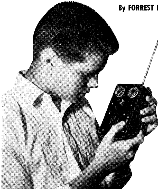
A neat, compact, two-transistor device, this portable intercom also functions as a broadcast band receiver.
